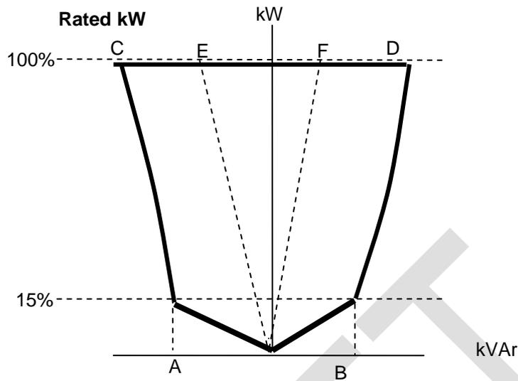
The figure above sets out the reactive power capability at the point of connection to the LV network.
